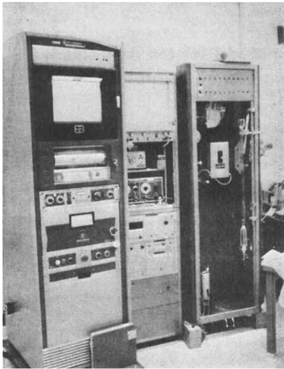
Fig. 1. Cahn balance thermogravimetric analyzer.
